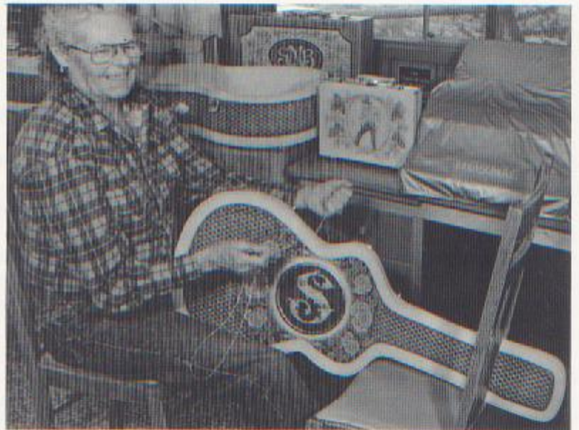
Ann Stohleman sewing the miter joint on the lid of the guitar case.
